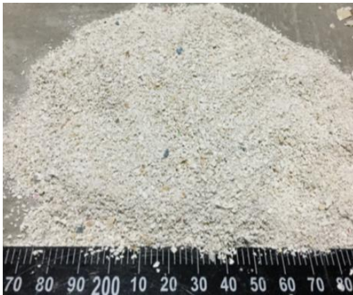
Fig. 5: View of fine grading PVC aggregate.
