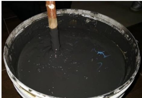
Fig. 3: Silica fume slurry.
